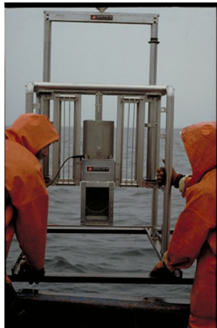
Figure 1. The sediment profile camera (right) is depth rated to 4,000 meters; the inset schematic (left) shows how the seafloor is photographed in cross-section.
